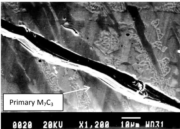
Fig. 1 – Scratching test of white chromium cast iron
