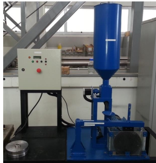
Fig. 2 – Test apparatus for the rubber wheel abrasion test
